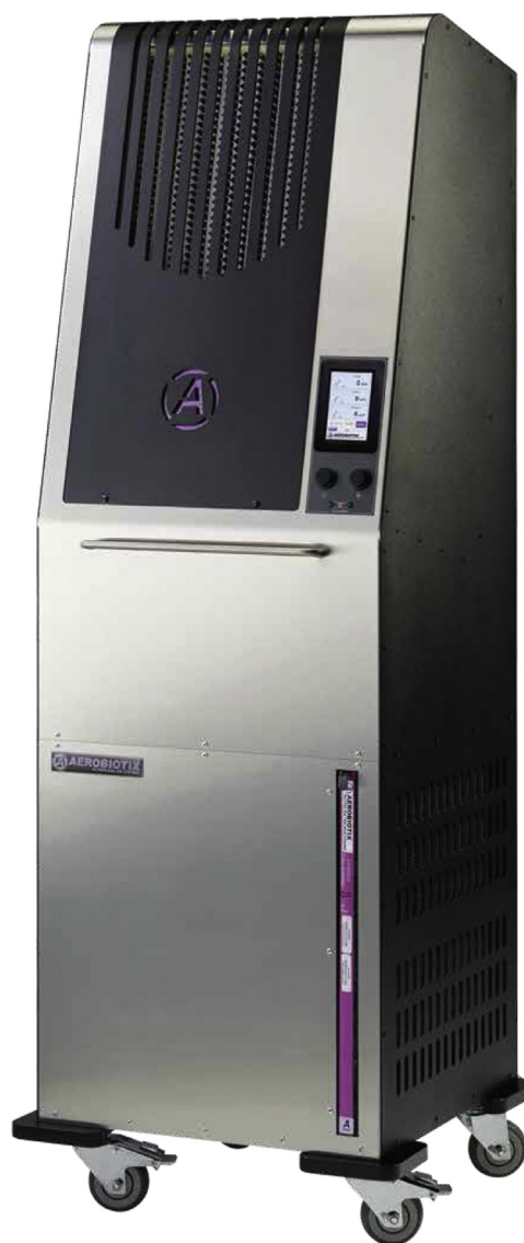
Fig. 1. The HUAIRS Illuvia unit is 46 × 46 × 150 cm and treats 12.8 cubic meters of air per minute, using a standard 115-volt outlet. The ultraviolet system is internal, preventing exposure to room occupants.
